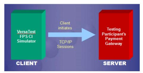
As the *client*, the VersaTest FPS CI Simulator mimics the default behaviour of the live FPS CI and initiates the TCP/IP sessions. The Testing Participant's Payment Gateway is configured as a *server* and 'listens' for the TCP/IP connections on the designated communication ports. The port allocations are defined in the FPS Hosted Accreditation Service Technical Set-up Guide.
